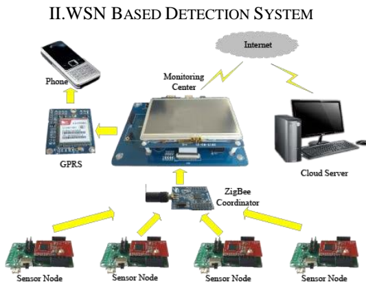
Fig. 1. The overall architecture of the monitoring system based on the WSN for the detection of gas leak.
