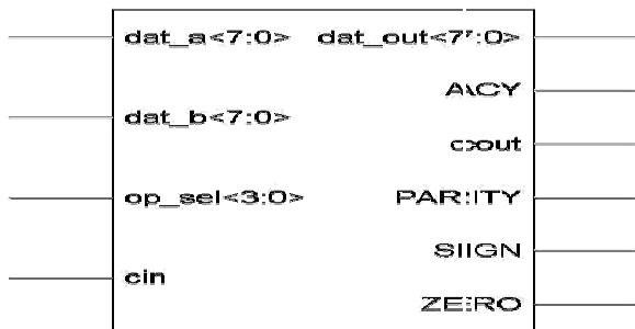
Figure 6. RTL Schematic of ALU
