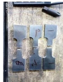
Dumbbell shape work pieces for tensile test
