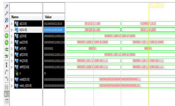
Fig 8: simulation result of ANT architecture when Baugh Wooley multiplier is used.
