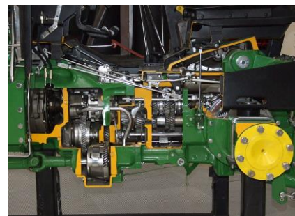
Tractor transmission with 16 forward and 8 backward gears
