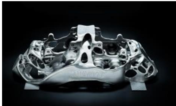
Bugattis 3D-printed brake caliper
