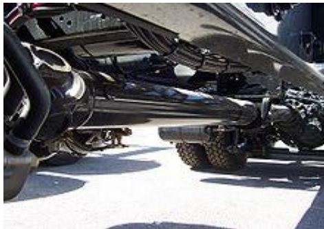
Fig:2.1 A truck double propeller shaft
