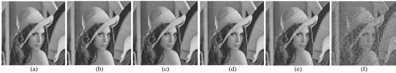
Fig. 27. Comparison of image lenna: (a) accurate adder; (b) SARA4; (c) SARA8; (d) SARA4-DAR2; (e) GDA; (f) RAP-CLA.
